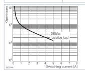
Electrical endurance Q1 / Q2. 2 A, 250 Vac, resistive load,  $10^5$  operations. 20/2 A, 250 Vac,  $\cos \varphi = 0.3$ ,  $10^5$  operations.
